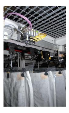
The data carriers are mounted on all products or containers and identify intermediate and end production stages during the entire production process.
